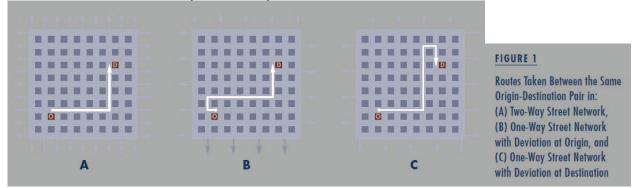
Figure 1: Illustration of the additional circuity of a one-way network compared to a two-way network
